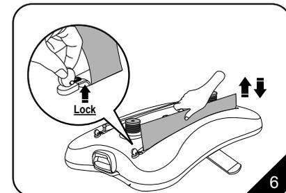
6. Pull the leading paper while lifting handle to lock in position.
