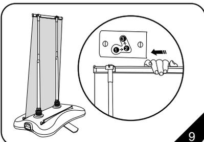
9. Aim two connectors in upper profile at ground hole in pole holder, shift to the right 7 hole, then raise till warhead out, advise operated to be by two person.
