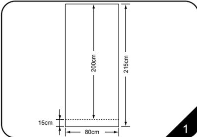
1. The overall dimension of the graphic is 80cm(wide) x 215cm (high). The visible overall height of the graphic is 80cm (wide) x 200cm (high). Please allow extra length for graphic insertion.
