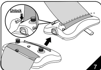
7. Adhere graphic to 3M on leading paper smoothly, then stick all around by transparent tape, then lift graphic and unlock by pressing the handle for rolling up graphic.
