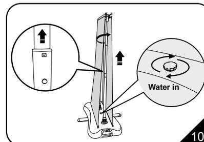
10. Raise the middle pole to the highest point, The graphic can be tightened by adjusting the pole. Then inject water into water base.
