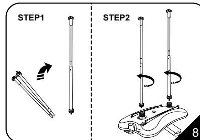
8. Unfold the pole and slip the pieces together to assemble it to a rigid pole. Attach vertical poles to the spring by screwing tightly, put warheads outward.
