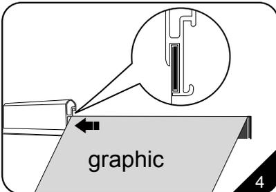
4. Take out the plastic piece from upper profile, and glue with the graphic, rotate 360 then insert into the profile as per above pic.
